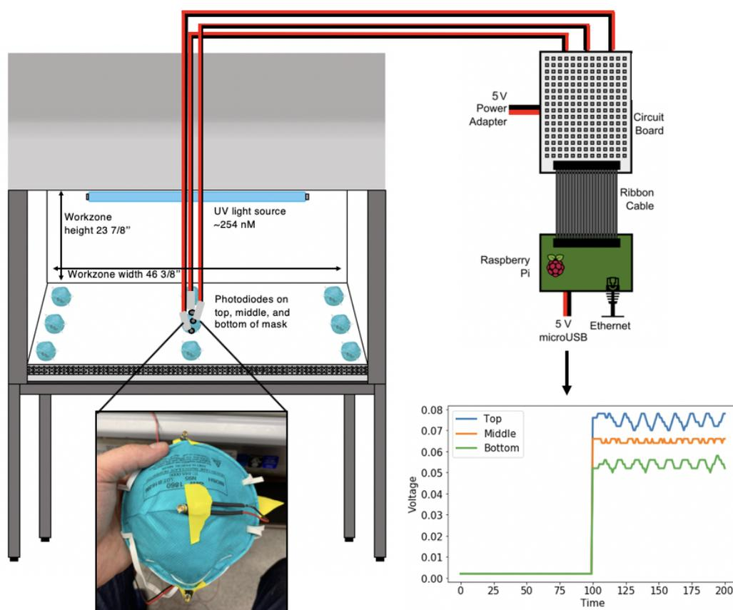
**Figure 1. Schematic of our process for measuring light intensity across the base of a BSC.** A photodiode was attached to the top (north), middle, and bottom (south) of an N95 mask, and the voltage of light that reached diodes was measured both with the UV light turned off and then on. This measurement was performed within each sector of a 3x3 grid at the base of the BSC workzone as illustrated.
