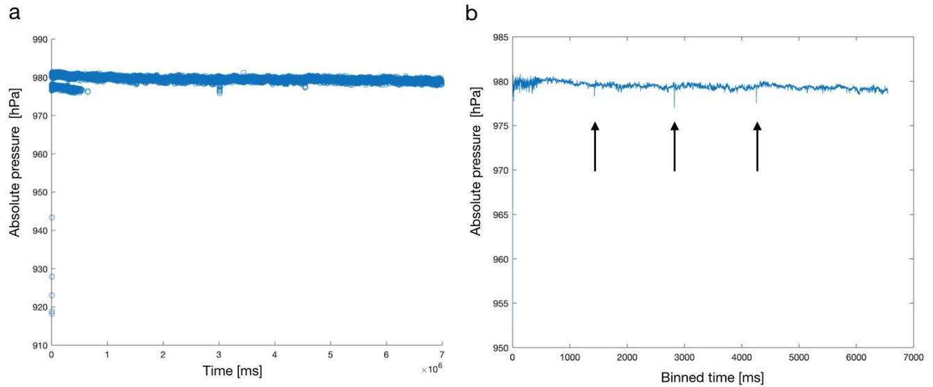
**Figure 2 - “Quasi-continuous” data recorded for a device.** We show an example of the data recorded for one of the three tested devices, namely the smartphone. Panel a: fitted data over time; panel b: fitted and downsampled absolute pressure data over time. Arrows indicate drop in the signal measurements.
