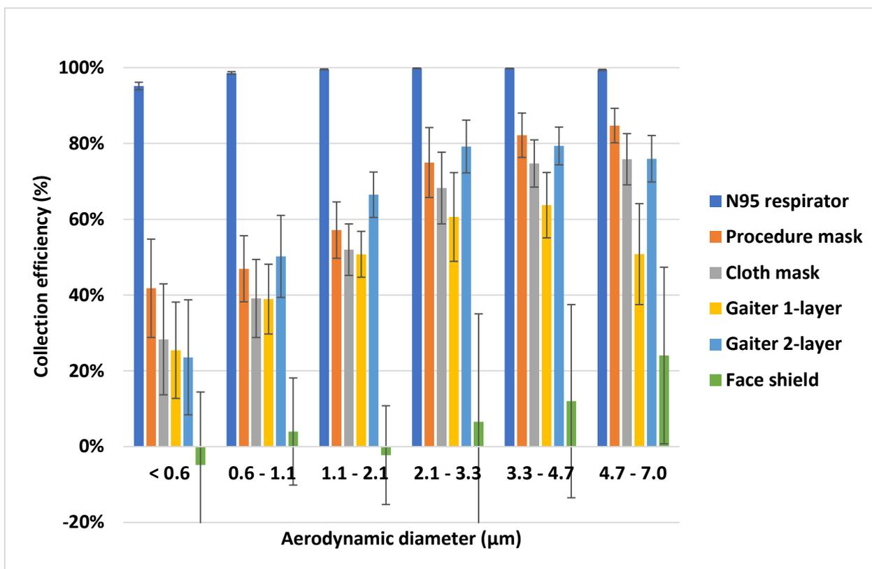
**Figure 3: Collection efficiency of face masks, neck gaiter and face shield.** The collection efficiency is the percentage of aerosol particles that were blocked by the face mask, neck gaiter or face shield compared with experiments without a device. The plot shows the means and standard deviations of the collection efficiency in each size fraction.
